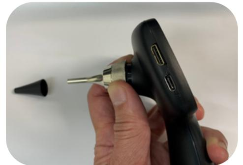
3. Fit the **speculum** over the tip camera.
